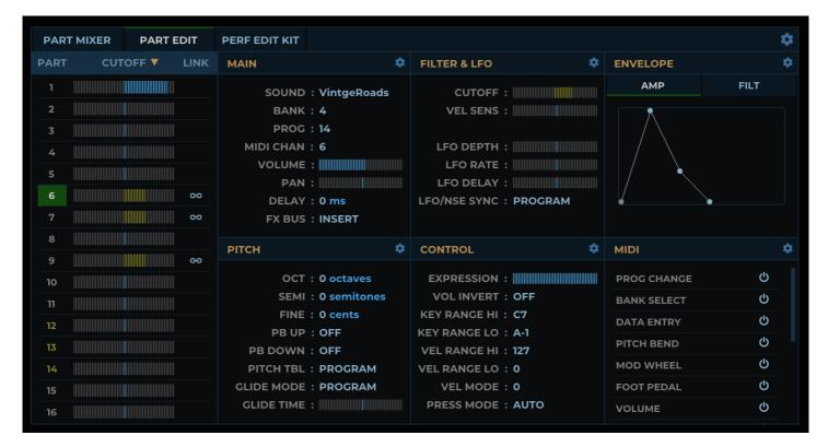
This tab allows editing of all parameters for a single part. A menu at the top right of the Part Edit section includes options to copy, link and unlink all part parameters, as well as an option to initialise the part.
