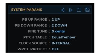
This section contains the system parameters found on the MR. Single system parameter change messages are not supported, therefore when editing a system parameter, a message will be sent containing all system parameters. This should be noted in case the system parameters on the hardware differ from those in the editor. It is advisable to sync the editor and hardware by clicking the request icon in the System Params section header before editing system params.
