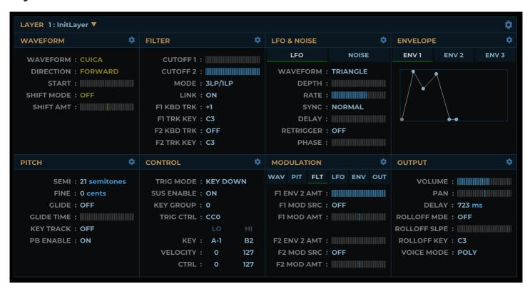
The main section of the Sound Editor is for editing the layer parameters. Select the current layer from the drop-down menu at the top left. A sound can have up to 16 layers. Set the number of layers in the <u>Sound Parameters (page 24)</u> section.
